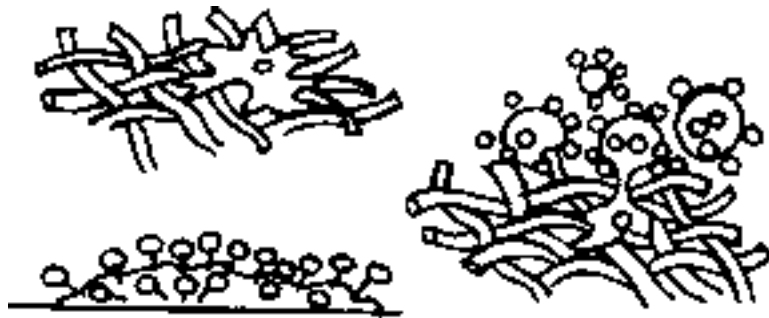
Fig. 27.5: Removal of dirt by detergents
